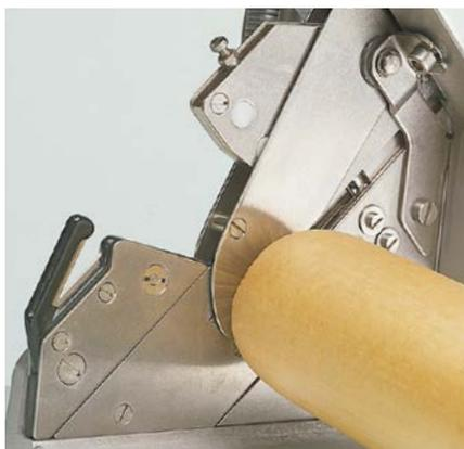
W-shaped "butt to butt" closures for natural casings.
